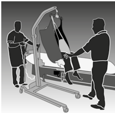
Figure 44 - A mobile hoist reduces the forces required to transfer a patient
