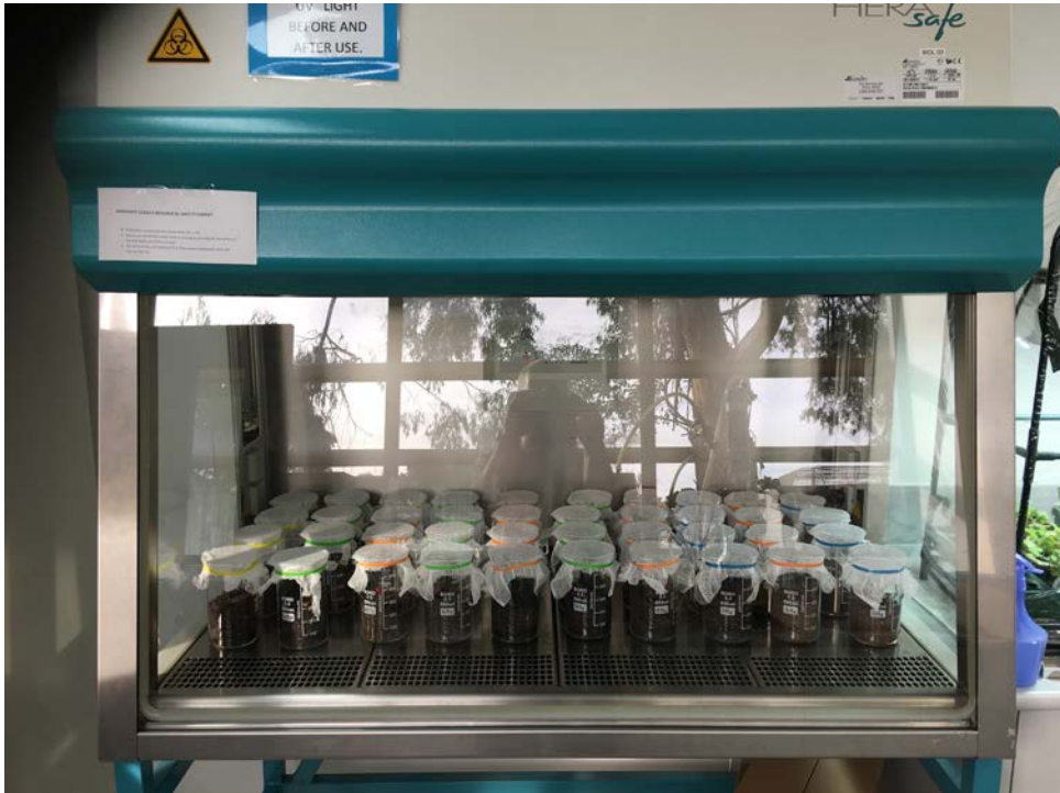
Figure 5. Fruit samples were added to 600 ml beakers containing 170g potting mix, covered with gauze, and then checked daily for emerging flies.
